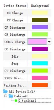
All the states supported by the device are displayed in color, which enables users to easily understand the current operating status or find the test channels for abnormal states when applying the device in large quantities.
