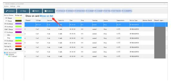
After a successful connection, the battery information will be displayed, including the current voltage, working current, test capacity, test time, work step number, working status, test status, temperature and equipment model.
