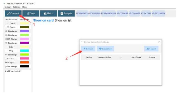
After installing the software, connect the instrument to the computer using a communication cable. Click the "Connect" button in the upper left corner of the interface, then click "Search". The ip address of the device will appear. Click "Connect" to control the instrument.
