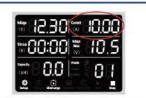
After the voltage is set, continue to press the black setting knob, the current bar flashes, and turn the black setting knob to set the discharge current.
