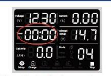
After setting the charging capacity, press the black setting knob, and the time display "00:00 "sets the rest time in the charging and discharging interval.
