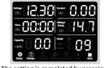
The setting is completed by pressing the red start knob. Set automatic jump work to complete charging--- pulse repair --- discharge --- charging
