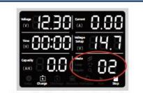
Press the black rotary knob, the mode selection bar at the bottom right flashes, and turn the black setting knob to set it to "02" mode.
