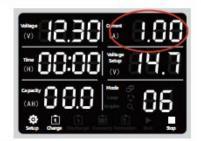
After setting the charging current, press the black setting knob to display "1.00 "and turn the black setting knob to select the charging cut-off current
