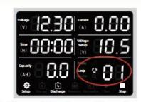
After the mode is set, press the cycle number at the bottom right of the setting knob to flash and rotate the black setting knob to select the number of cycles (1-50 times)
