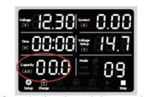
after setting the pulse repair time, press the black setting knob, the accumulated capacity display "00.0 ", rotate the black setting knob, and set the third step charging capacity to keep "00.0" as direct charging. if it is necessary to set the charging capacity, the setting capacity must be less than the nominal capacity.
