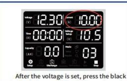
After the voltage is set, press the black setting knob, the current bar flashes, and turn the black setting knob to set the discharge current.
