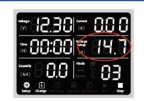
Press the black setting knob, the voltage column flashes, and turn the black knob to set the cut-off voltage for the second step of charging.
