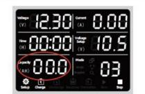
after the charging cut-off current is set, the accumulated capacity displays "00.0 "and rotates the black setting knob to set the charging capacity in the second step to keep "00.0" as no setting. if the charging capacity needs to be set, the capacity must be less than the nominal capacity.
