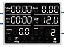
Charge and discharge current can be arbitrarily adjusted Charging current adjustment range 0.5-6A Discharge current adjustment range 0.5-10A Mode code
