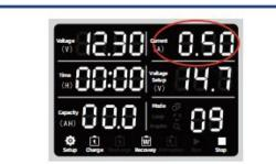
After setting the discharge current, press the black setting knob to enter the second step, and the pulse repair current displays "0.50 "to set the pulse current
