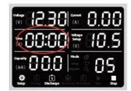
after setting the charging cut-off current, press the black setting knob, and the time display "00:00 "sets the rest time in the charging and discharging interval
