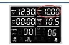
After the discharge cut-off voltage is set, press the black setting knob, and the current bar flashes and rotates the black setting knob to set the discharge current
