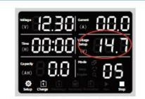
Press the black setting knob, the voltage column flashes, and turn the black knob to set the cut-off voltage for the second step of charging
