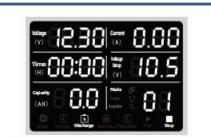
After setting the discharge current, continue to press the black setting knob, and press the red starting knob after the current display 00.0 is set.
