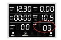
Press the black setting knob, the mode selection bar at the bottom right flashes, and turn the black setting knob to set it to "03" mode.
