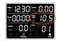
After the mode is set, press the voltage setting column of the setting knob to flash, and turn the black setting knob to set the discharge cut-off voltage.
