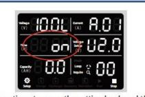
continue to press the setting knob and the time setting column "on "flashes (turn on or off the fan detection function, normally on by default)
