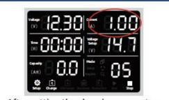
After setting the charging current, press the black setting knob to display "1.00 "and turn the black setting knob to select the charging cut-off current.
