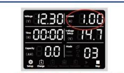
After setting the charging current, press the black setting knob to display "1.00" and tum the black setting knob to select the charging cut-off current.
