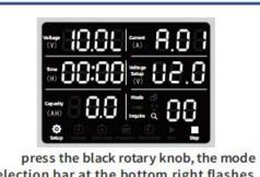
selection bar at the bottom right flashes rotate the black setting knob to set to "00" mode and press the button
