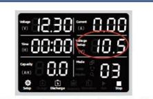
Press the voltage setting column of the black setting knob to flash, and turn the black setting knob to set the discharge cut-off voltage.
