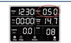
After the voltage is set, press the black setting knob, the current bar flashes, and turn the black setting knob to set the pulse charging current.
