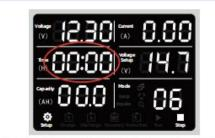
after setting the discharge current, press the black setting knob, and the time display "00:00 "sets the rest time in the charge and discharge interval
