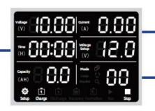
Charge and discharge current range can be arbitrarily adjusted Charge current adjustment range0.5-6A Discharge current adjustment range 0.5-10A Mode code
