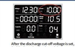
press the black setting knob, and the current bar flashes and rotates the black setting knob to set the discharge current.
