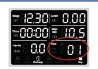
Press the black rotary knob, the mode selection bar at the bottom right flashes, and turn the black setting knob to set it to "01" mode.
