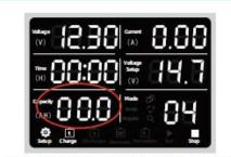
after setting the discharge current, the accumulated capacity displays "00.0" and rotates the black setting knob to set the third step charging capacity to keep "00.0" as no setting. if the charging capacity needs to be set, the capacity must be less than the nominal capacity.
