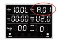
after the mode is set, continue to press the current setting column "A.01" of the setting knob to flash (the address of the lower channel of the networking equipment)
