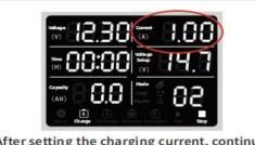
After setting the charging current, continue to press the black setting knob, the current bar displays 1.00, and rotate the setting knob to select the cut-off current.
