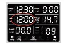
After setting the pulse current, press the black setting knob, and the time display "12:00 "rotates the black setting knob to set the pulse repair time.
