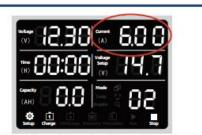
After the voltage is set, continue to press the black setting knob, the current bar flashes, and turn the black setting knob to set the charging current.
