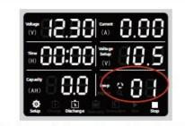
After the mode is set, press the cycle number at the bottom right of the setting knob to flash and rotate the black setting knob to select the number of cycles (1-50 times)
