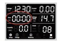
After the setting is completed, press the red start knob. Set automatic jump work to complete pulse repair.
