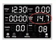
Press the voltage setting column of the black setting knob to flash, and turn the black setting knob to set the charging cut-off voltage.
