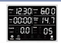
After the charging cut-off voltage is set, press the black setting knob, and the current bar will flash and rotate the black setting knob to set the charging current.
