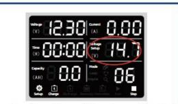
Press the voltage setting column of the black setting knob to flash, and turn the black setting knob to set the charging cut-off voltage.
