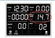
After the mode is set, press the voltage setting column of the setting knob to flash, and turn the black setting knob to set the charging cut-off voltage.
