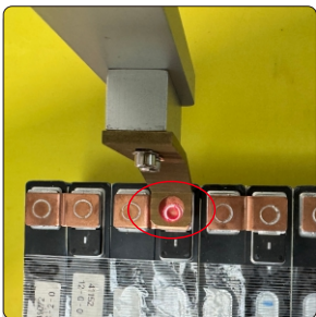
10.Make sure the red light position is on the welded object and is not blocked by the limiter.
