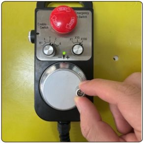
6.Use the locator handwheel to move the laser welding head to the welding position.
