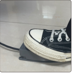
15.Press the foot pedal switch, and the machine starts to emit laser for welding.
