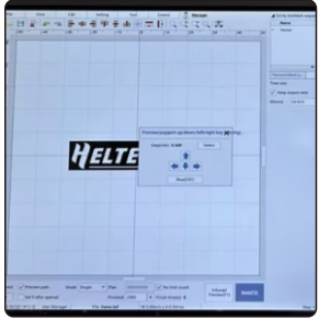
9.Adjust the red light path according to the size of the graphic.
