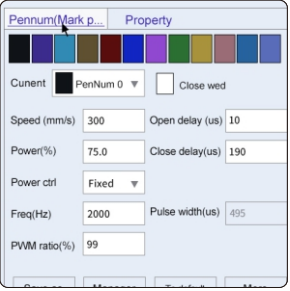
13.Set the welding parameter in "PenNum/Mark parameter".(Please refer to the recommended parameter setting table on the following page.)
