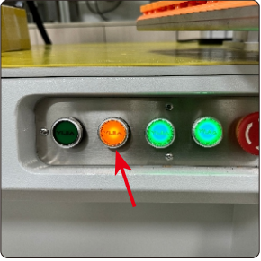
14.Press the yellow button to allow laser emission after confirming the red light position and welding parameters.
