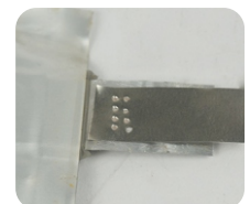
3. Check the spots' reliability. Finish spot welding.
