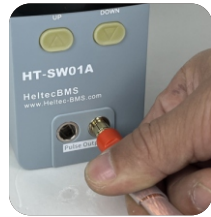
③ Insert the mobile welding pen and make sure the connection is solid.
