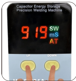
1. Starting up— Press the "▲/▼" button at the same time to switch on the spot welder.
