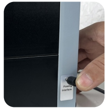
① Plug the power output plug into SW01A spot welder power connection port.
