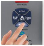
2.Press the "START" key after switching to the discharge mode, and the machine will be in discharge equalization.the corresponding indicator lights will remain on until the discharge equalization is finished, the indicator light will turn off
