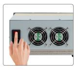
1.Power-up:Press the " O "button at the back of the machine to turn on the main power switch.
