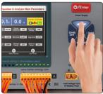
6.During the equalization process, pressing the "STOP" button can stop the equalization .
