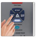
2.Press the "CHG ON" button to start the charge equalization mode according to the set parameter.
