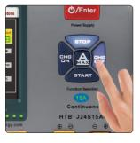
3.Press the "CHG OFF" button to stop the charge equalization mode.
