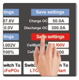
4.Set the "equilibrium limit" parameter based on the voltage status of the battery pack. the machine will automatically turn on discharge equalization when the voltage exceeds the set value
