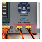
4. The total positive and negative poles of the battery need to be connected to the machine (left interface), and the charger needs to be connected to the input terminal (right interface) in charging mode.
