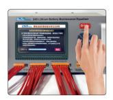
3.After turning on the main power switch, briefly press the " $\mbox{\it 0}$ " button to start the control display screen.
