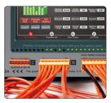
5.The corresponding string number indicator light will flash in discharge equalization mode, and the light will go out when the equalization is over.
