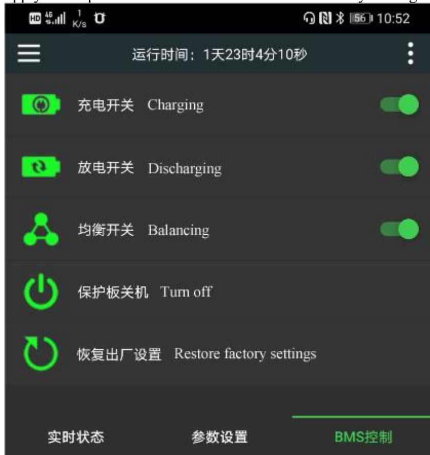
The BMS control page
