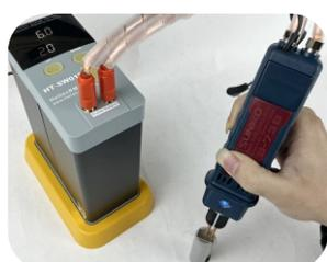
Attach welder to base to prevent movement during welding process.
