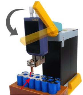
The distance between of the welding needle and battery is 4-9mm.
