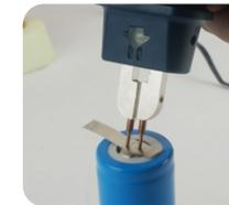
2. Hold the welding pen and apply a certain pressure to the object's surface (e.g. nickel strip) simultaneously. Automatic welding begins after about 20ms.
