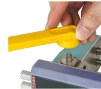
1. Insert the welding head into the corresponding socket.
