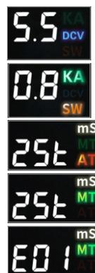
The charging voltage of the spot welder is 5.2~5.8.
