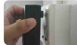
① Plug the adapter into an AC 100-240 volt wall socket to charge the machine.
