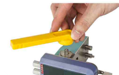
1. Insert the welding head into the corresponding socket.
