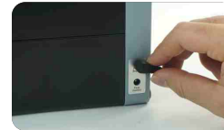
② Plug the power output plug into 801H spot welder power connection port.
