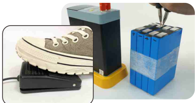
3. Hold the spot welding pen and press the welding needle tightly, step on the wire-controlled foot switch to trigger spot welding, and observe and check that the real-time welding current on the display should be within the range of 2.8~3.3KA (2800~3300A).
