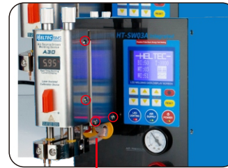
Loosening the pneumatic weld head screw to remove the weld head
