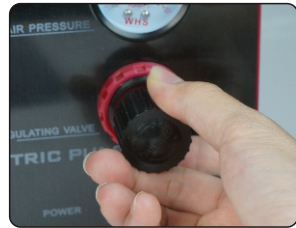
Air pressure adjustment knob
