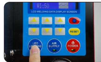
Press the "LED" key, turn on the lighting device
