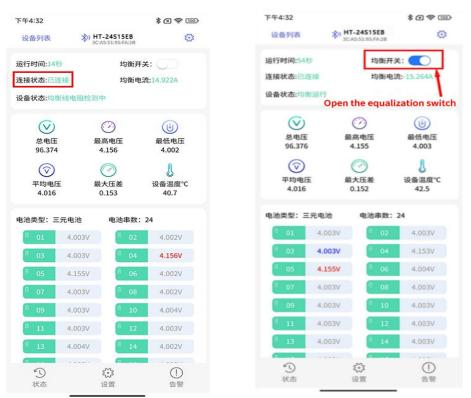
Thirdly, according to the battery type and strings, change the parameters( A password is required to access the settings for the first time) As shown in the picture below.
