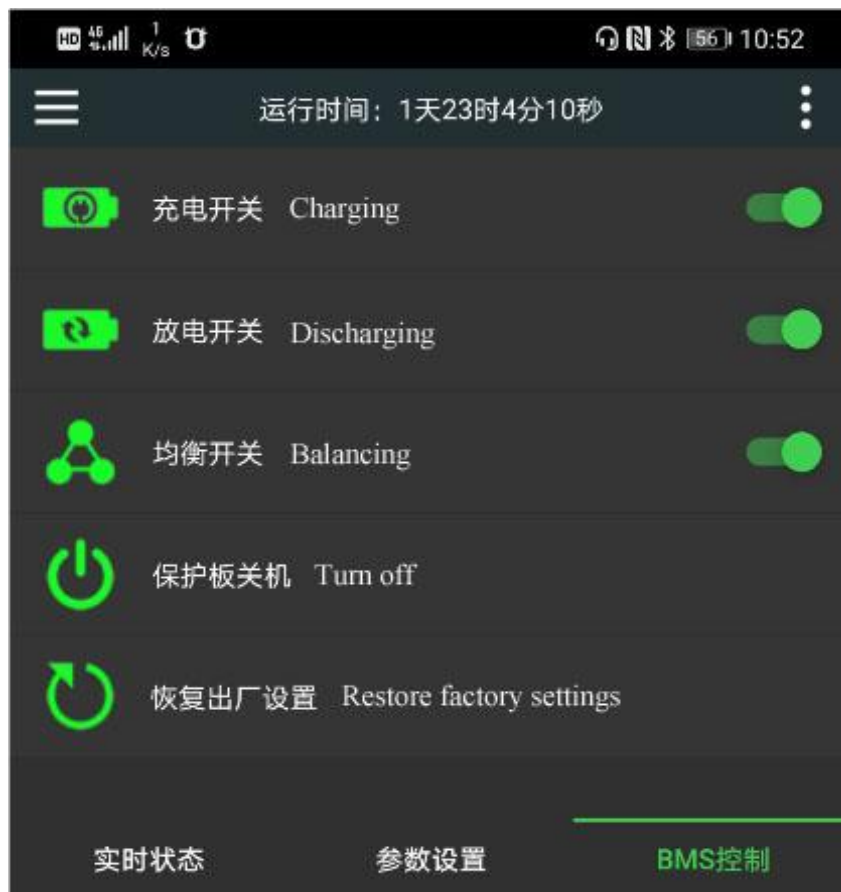
Figure 26. The BMS Control Page
