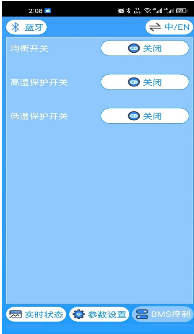
Figure 11. BMS Control Page
